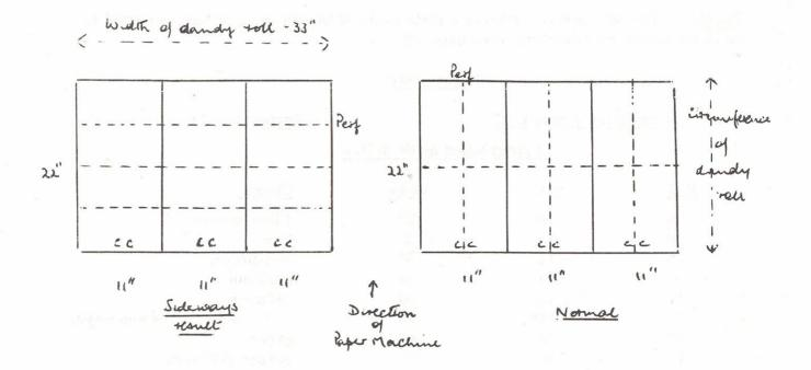
Each division of the original sheet, when cut, gives a smaller sheet of  $11 \times 5\frac{1}{2}$  inches. When the sub-divided sheets of example A are printed they would have to be turned through 90 degrees before being fed into the printing machine; thus the watermark is then 90 degrees out of true i.e. sideways.
